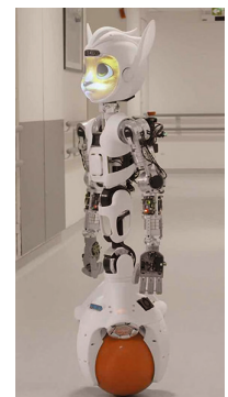
Figure 2.3 The Mirokai robot by Enchanted Tools, France. It combines omnidirectional navigation with two robot arms and a back-projected face. (Source: Enchanted Robots)
