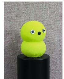
Figure 2.7 Keepon (2003–present), a minimal social robot developed by Hideki Kozima. The robot was later commercialized as an affordable toy. (Source: Hideki Kozima, Tohoku University)
