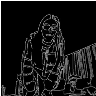
Figure 3.18 Canny edge detection of a user operating the buttons on a robot.
