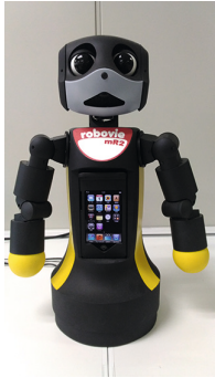
Figure 4.14 Robovie MR2 (2010) is a humanoid robot controlled through a cell phone.
