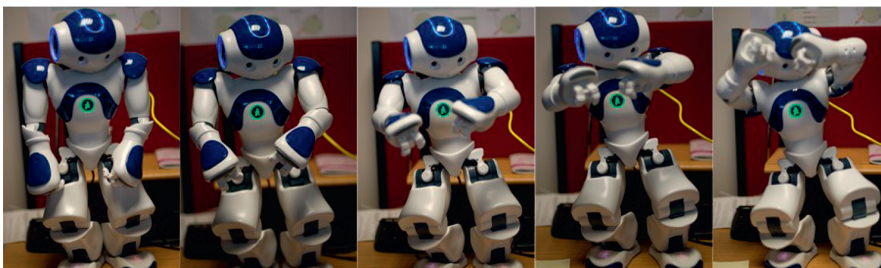
Figure 6.8 A Nao robot (2008–present) using body postures to express emotions, morphing between sad (left) and fearful (right). (Source: Beck et al. (2010))
